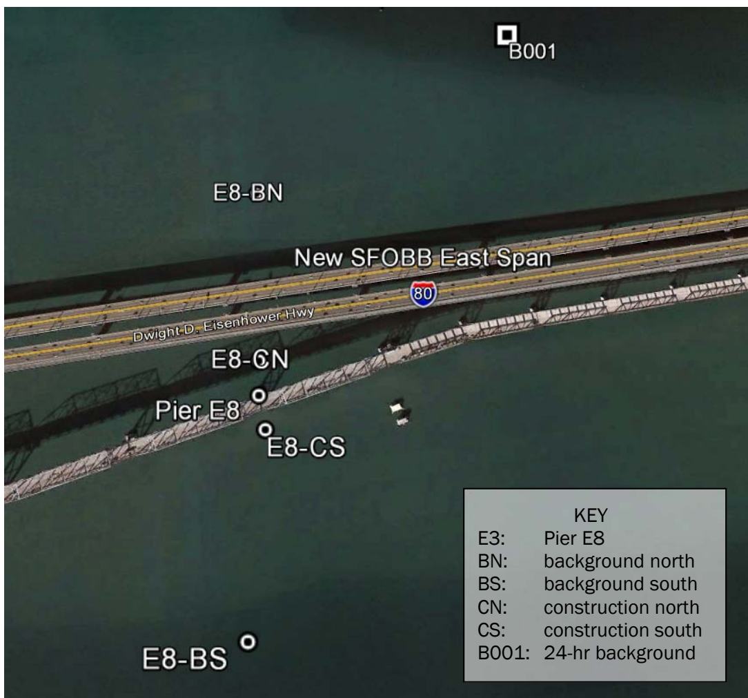
Figure 2-1. Example of approximate water quality monitoring sites for Pier E8 in-water activities.
